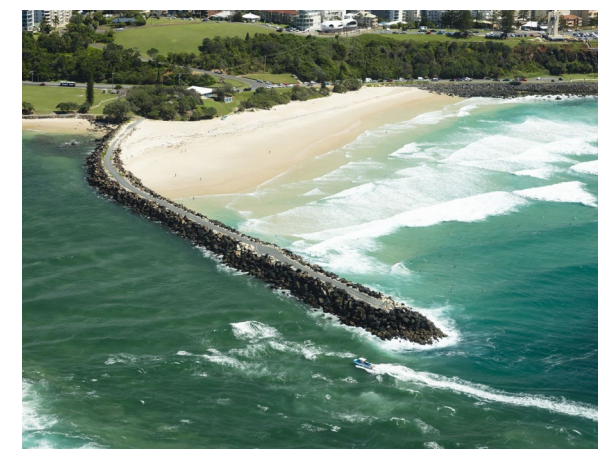
Figure 5b: These two images of Duranbah in northern NSW show the effects of cross-shore sand transport. In the left image (March 2018), due to generally calm conditions, cross-shore transport has created a wide beach. The right image (October 2019) illustrates the effect of cross-shore transport under larger wave conditions – sand has been removed from the beach and the width has been reduced. Source: Tweed Sand Bypassing
