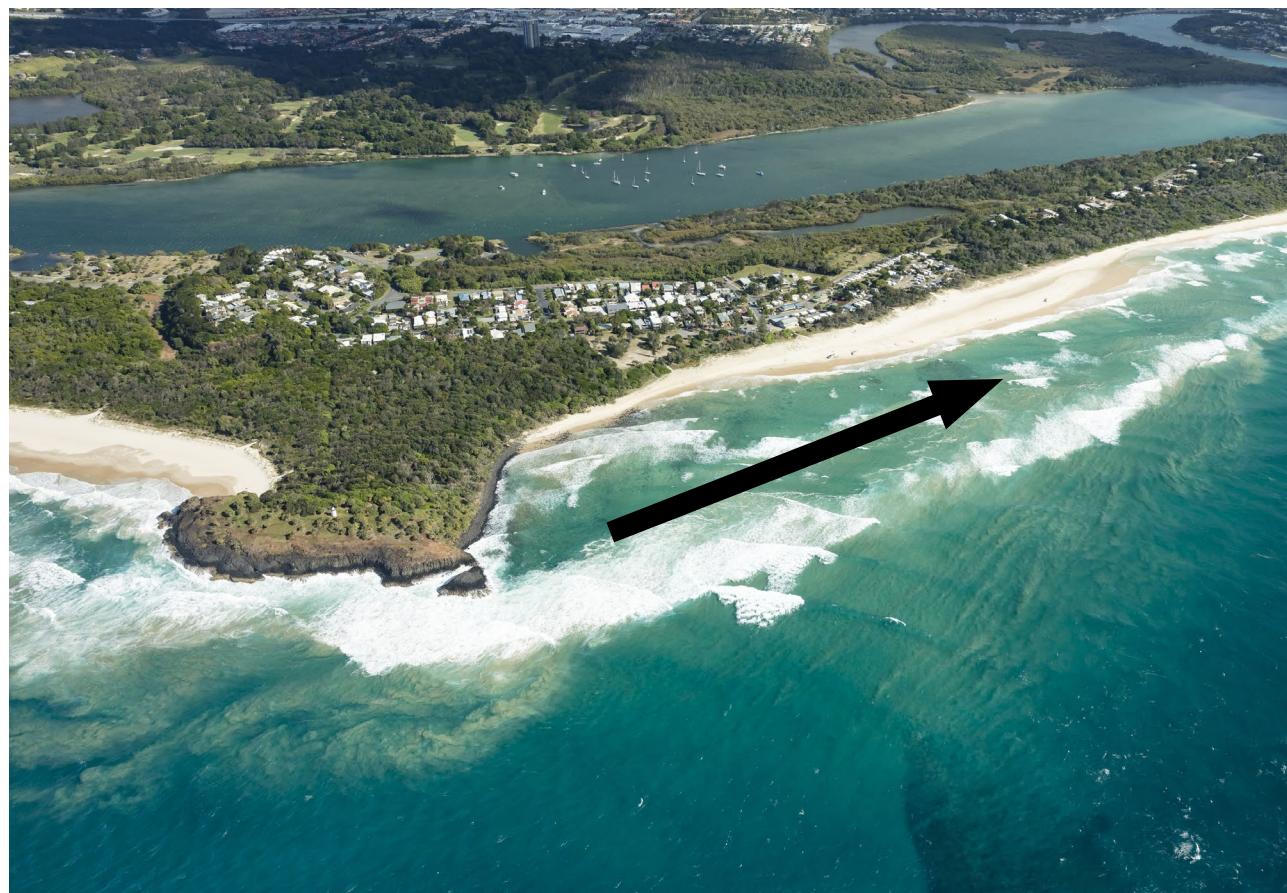
Figure 9: Longshore sand transport on Letitia Spit.
