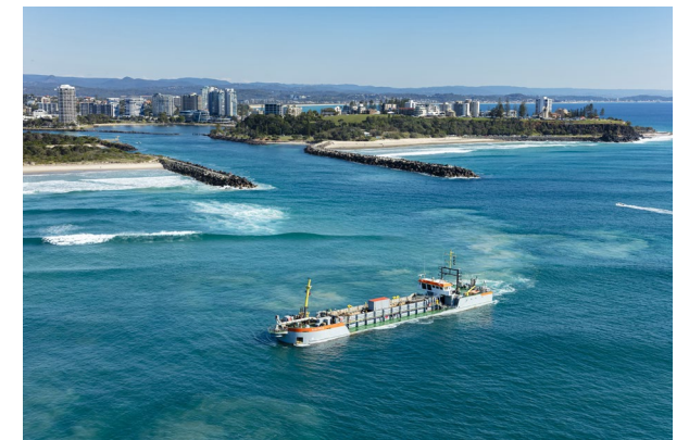
Figure 8: Tweed Sand Bypassing dredge, removing sand from the Tweed River entrance. Source: Tweed Sand Bypassing
