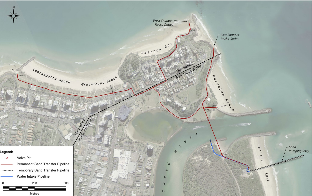
Figure 10: Map showing the sand pumping infrastructure. Source: Tweed Sand Bypassing
