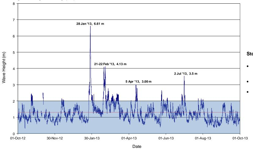
Note: The significant wave height is defined as the average height of the highest one-third of waves recorded over a period of typically 15 minutes.
