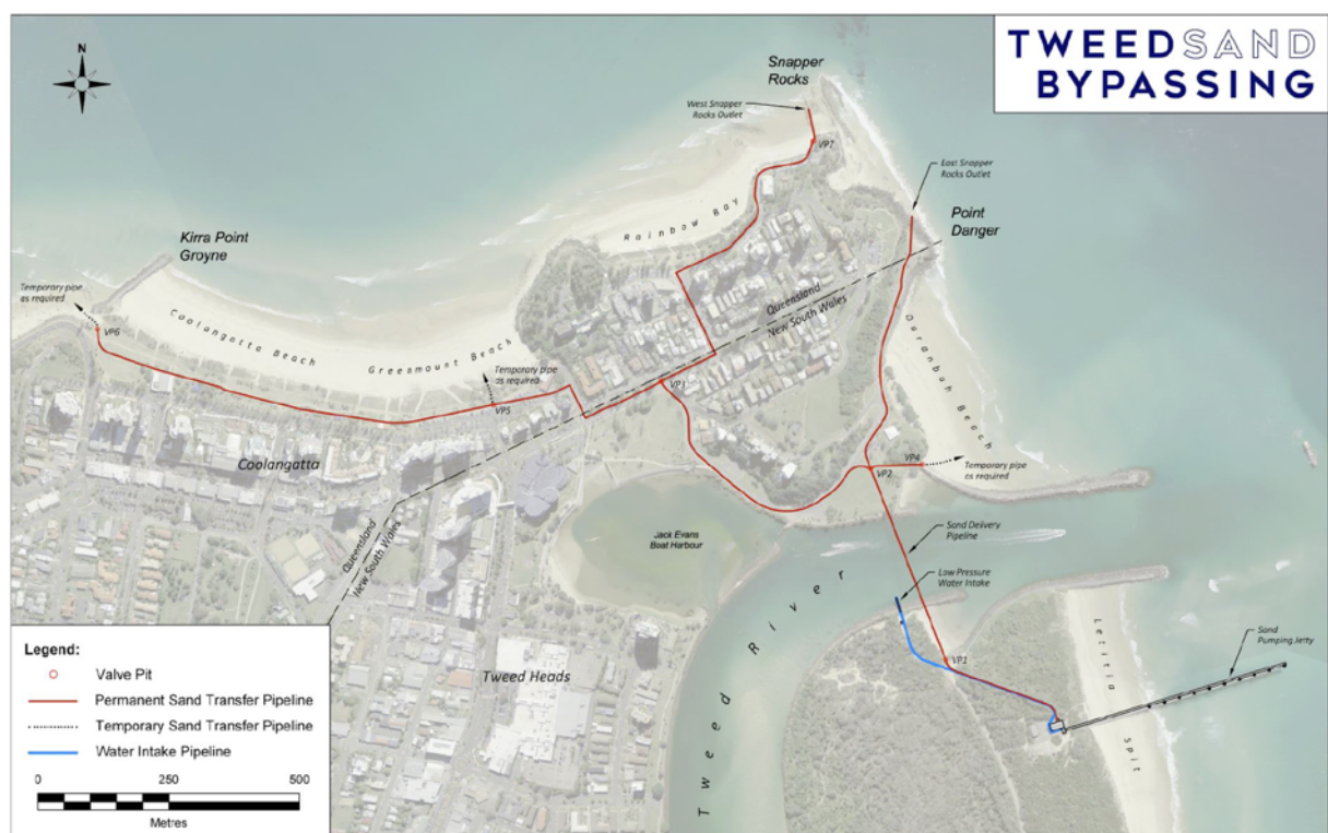
Figure 1.1 Fixed sand bypassing system (TSB, 2021)
