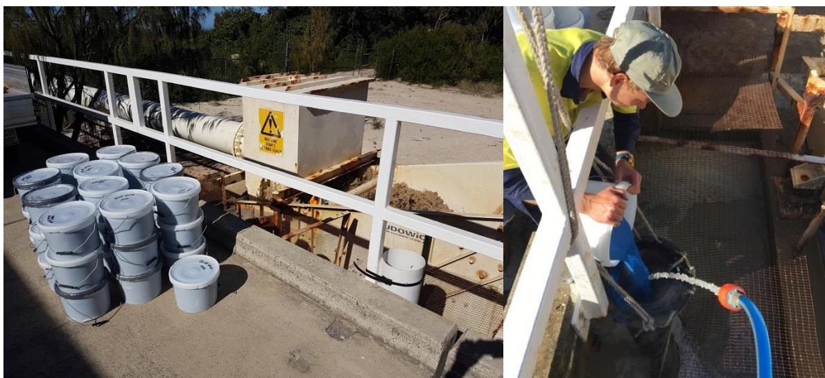
Figure 5: Southern end of slurry tank at the Letitia Spit jetty where the blue tracer material was injected (photo credit: Heiko Loehr/ Isaac Smith).
