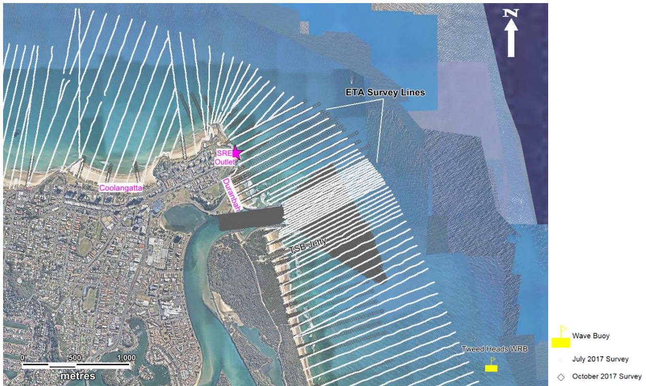
Figure 14: Map showing Tweed Heads WRB location and survey profiles (ETA lines) captured during study period.
