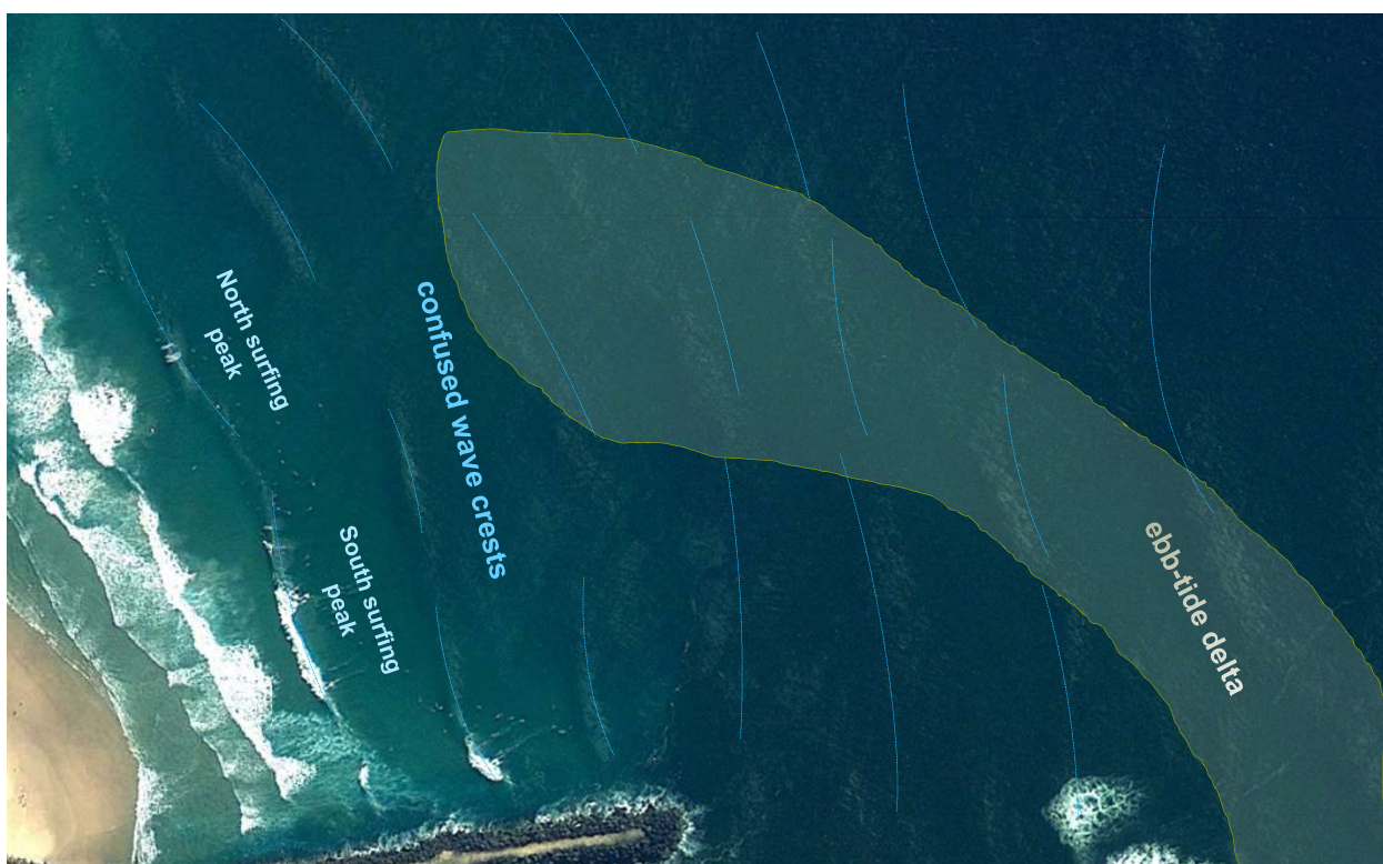
Figure 15 'Confused' wave crests in the lee of the Tweed River entrance bar. Two distinct peaks can be seen to be breaking along the 'Middle' section with several surfers centred on the breaking point of each (source: Google Earth 30 April 2009)
