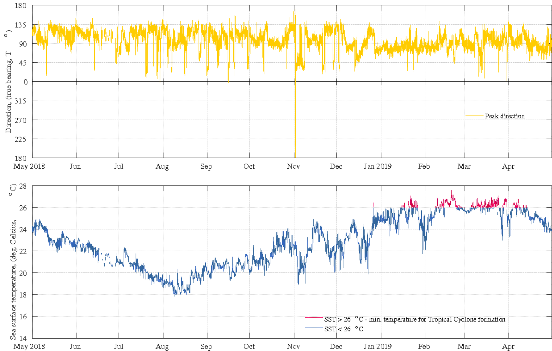
Figure 3.8: Tweed Heads Waverider buoy – Sea surface temperature and peak wave directions
